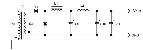
Figure 3. Schematic of the Two-Stage Output Filter
