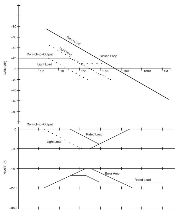
Figure 4. Compensation Bode Plots for the Example
