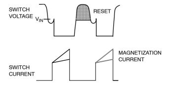
Figure 2. Power Switch Waveforms
