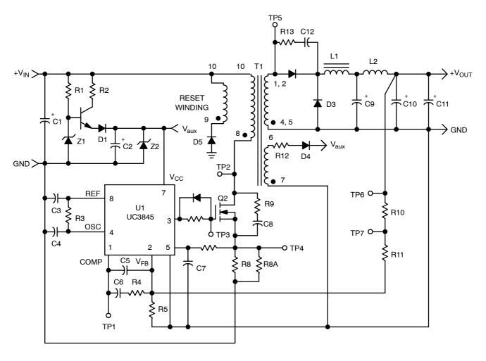
Figure 5. 112 Watt, One-Transistor Forward Converter
